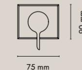
SMART BOX - Universal and quick installation for 1 way mixer with a Ø35 mm. ceramic cartridge and 1/2" connections. The 3 bar pressure is 22,1 L/min. 2 mufflers and a 1/2" plug included.
